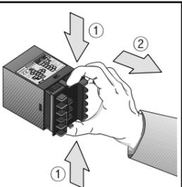
To select the input mode it is necessary to detach the housing. Before performing the operation always make sure that the device is powered OFF! Removing the housing should be carried out in two steps shown in the drawing. First press gently the two clips on the back side of the device. Select the desired input mode with the help of the SW1 and the SW2 pins and the jumpers on the circuit board. After setting the jumpers, replace the housing to the device.
