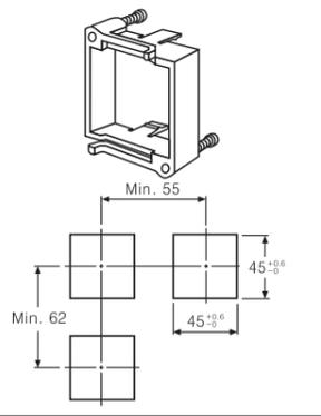
Using the optional PAM-500-0 front panel adapter the 48x48mm sized unit can be mounted to an existing 96x48mm cut-out hole. In case of using the front panel adapter, the width of the mounting-plate is 3-5 mm.
