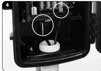
5. If using a 16-30VDC mains charger then plug this into the socket shown in the picture below. Alternatively, the charger may be wired into the solar panel screw terminal block (*to the left of the socket*).
